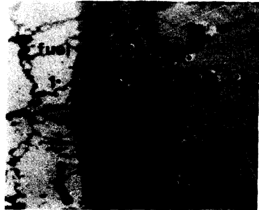
Fig. 12 SEM Back Scattered Electron Image of Clad-Fuel interface in Location B on Fig. 10.
