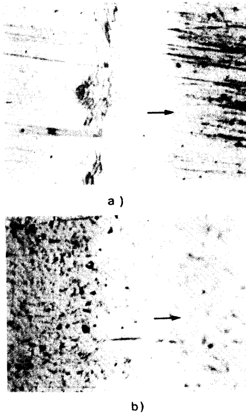
Photo. 4. Pictures of wear scars varying with coating film thickness. (2.5Kgf, 1.0m/sec, 31m, Arrows indicate sliding direction) a)TiN 1 μm × 300 b) TiN 3 μm × 300
