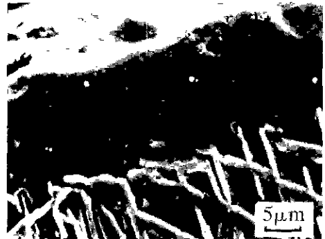
Fig.10. Cross sectional morphology of Mn-Zn ferrite excessively oxidized in air at 1000°C for 100 hrs.
