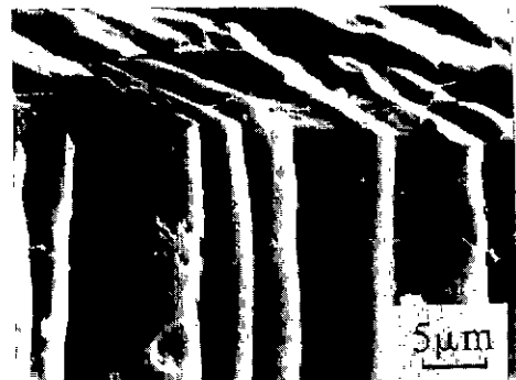
Fig. 4. SEM micrographs showing the morphology of lath-type hematite precipitated within Mn-Zn ferrite by oxidation in air at 1000°C for 24 hrs.
