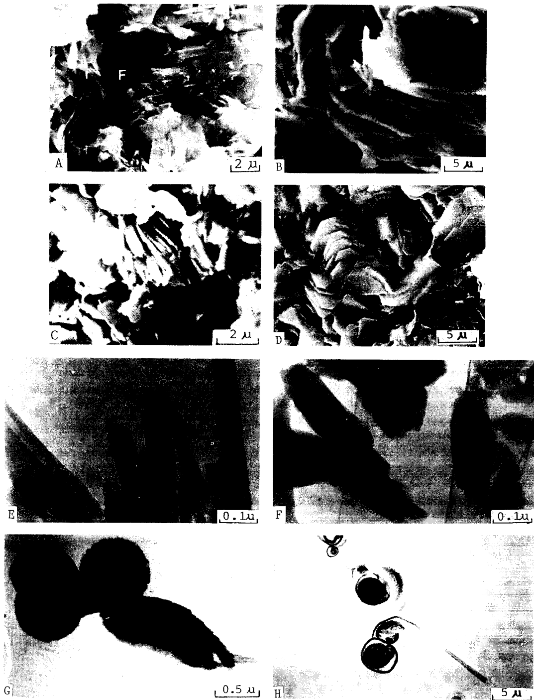
Fig. 3. (A-D) SEM photographs. (A) Sericite (muscovite) (S) on feldspar (F). (B) Flaky sericite. (C) Dickite in book-form. (D) Flaky pyrophyllite. (E-H) TEM photographs. (E) Long tubular form of 10 Å-halloysite. (G) (H) Spherulitic forms of 10 Å-halloysite.
