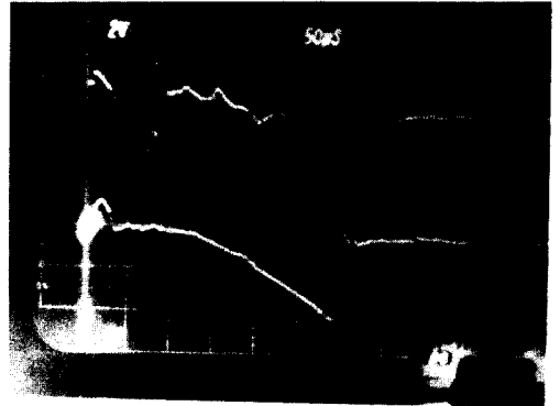
Photo. 5. Voltage profile of the trigger plate (upper) and spark gap (lower).
