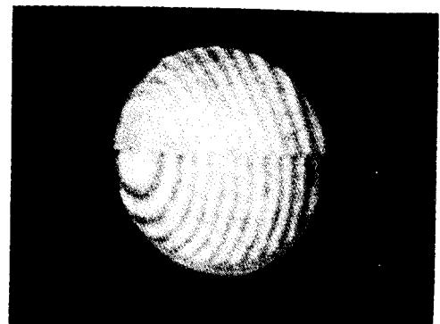
Fig. 5. Interference fringe pattern in binary phase modulation
