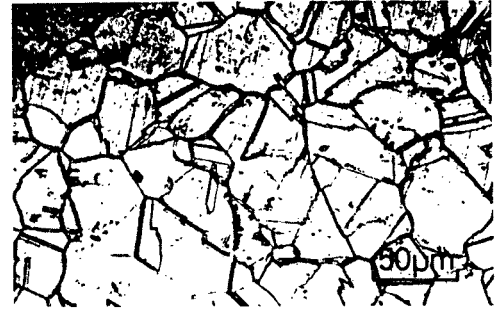
Fig. 1 Microstructure of type 304 stainless steel
