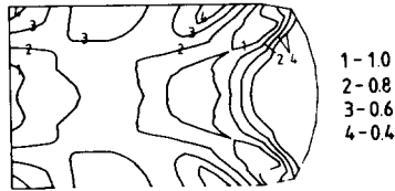
Fig. 18 Distribution of effective strain rate for plane strain forging (50% height reduction, die speed 10mm/sec)
