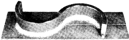
Photo. 4 Example of seam tracking at S-shaped workpiece
