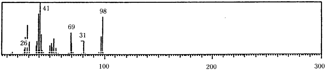
Fig. 3. Mass spectrum of 3-furan methanol
