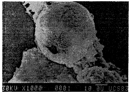
Fig. 12. Hollow sphere exhibiting a surface shrinkage hole
