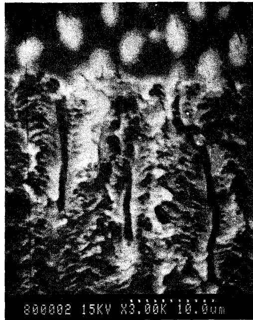
Fig. 12. Fractured surface treated with 3% H_2O_2 in Fig 11. \times 3000 .
