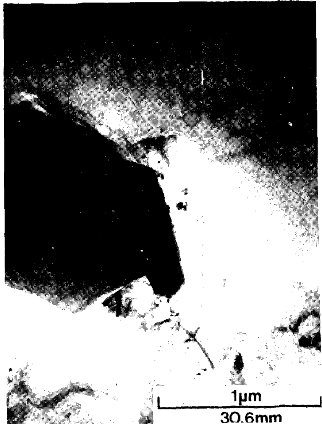
Photo. 6 TEM view of TiAl 3 or TiB 2 in grains, grain refined with AlTi5B1 master alloy.
