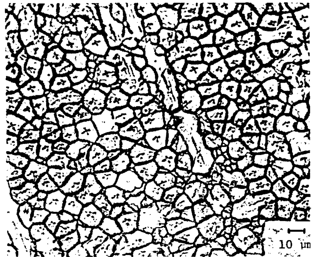
그림 8. The spherical morphology showing dark colored solute-rich crosses in the center of each element, surrounded by a solute-poor region which gradually darkens toward the edge. The sample was supercooled 20K before quenching in molten lead(after McDevitt and Abbaschian 19) ).
