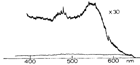
Fig. 4. The LaOCl host emission, incident light is UV (230-270). The peaks at 450~500 nm are xenon characteristics and the broad peak at 550 nm is 2nd order diffraction of monochromator.
