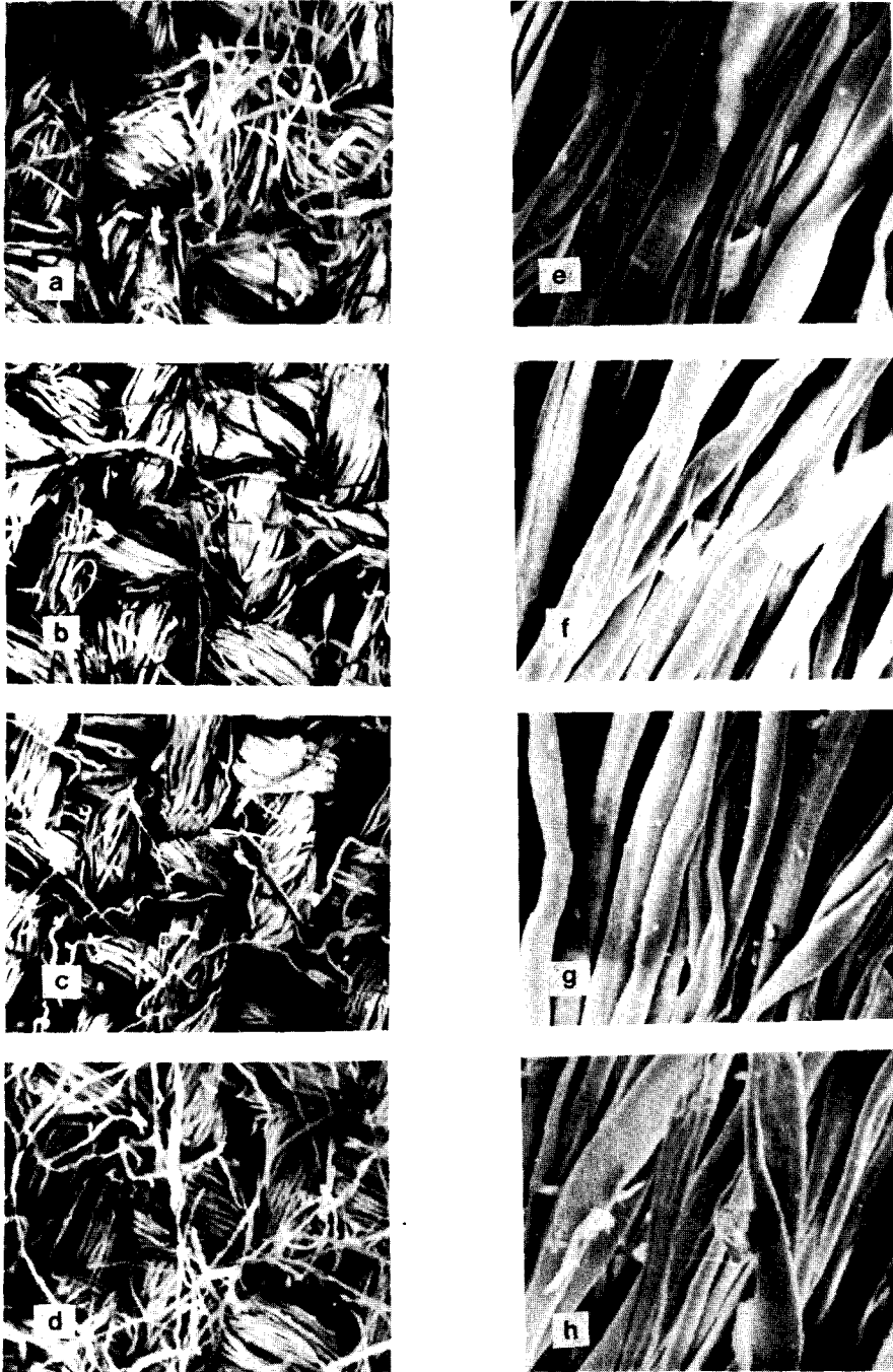
Fig. 4. SEM photographs of abraded surface of CF by worsted fabric abradant (900 rubs). (a) CF 1 (43×), (b) CF 2 (43×), (c) CF 3 (43×), (d) CF 4 (43×), (e) CF 1 (430×), (f) CF 2 (430×), (g) CF 3 (430×), (h) CF 4 (430×).
