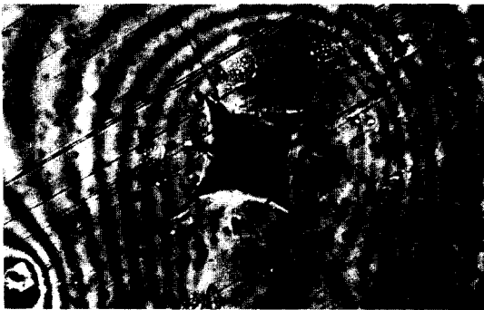
Fig.3. Micrographs showing Vickers indentation damage at 10 N in (a) the unworn and (b) the worn area of the same specimen as shown in Fig. 2-(b). Note that the length of the cracks in (a) and (b) is approximately same.
