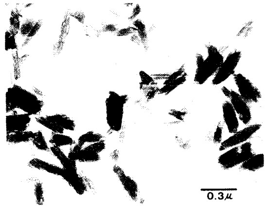
Fig. 2. Transmission electron micrograph of halloysite in common kaolin.
