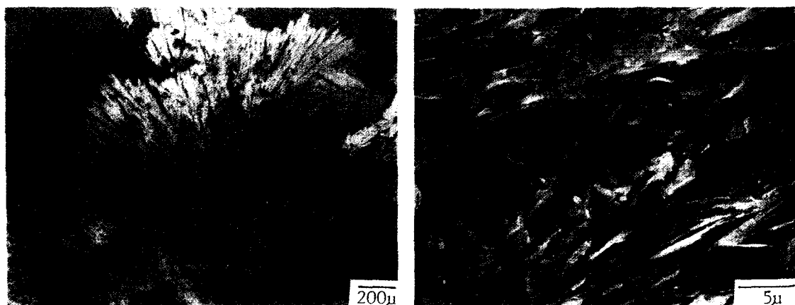
Fig. 1. The natural Ca-busserite-rancieite flakes from Dongnam mine, Korea. (A) Radiating or subparallel groups of flaky crystals in polished section. Open nicols. (B) Flaky crystals under SEM.
