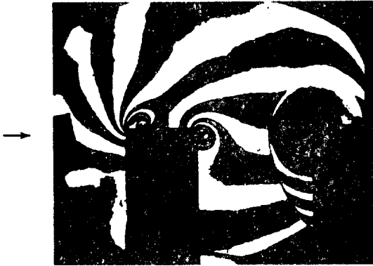
Fig. 7 Vortex generation at the edges of a block after a shock wave from the left hits the block(Mach-Zehnder interferogram by H.U. Hassenpflug, Aerodynamisches Institut, Aachen)
