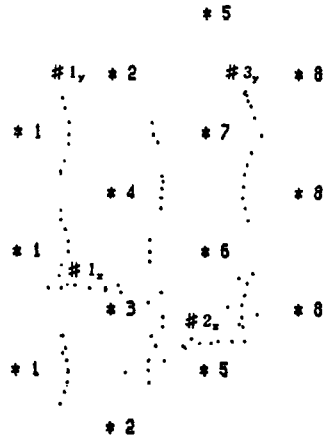
Fig. 9. Distribution of AE events from pencil break vs sensor location using 8 channels on model vessel of SS4l
