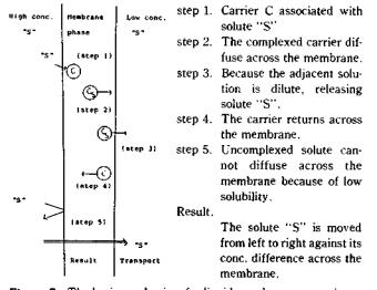
Figure 3. The basic mechanism for liquid membrane separation.
