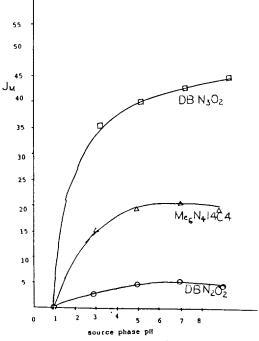
Figure 4. Plot of flux value of Cu<sup>2+vs.</sup> source phase pH.
