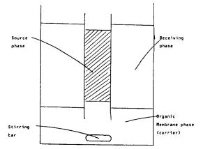
Figure 1. Bulk liquid membrane system.
