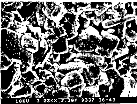
Fig. 7. SEM photograph of prepared Ba_2Ti_9O_{20} powder by coprecipitation method. (in air : 1400^\circ C , for 5 hrs).
