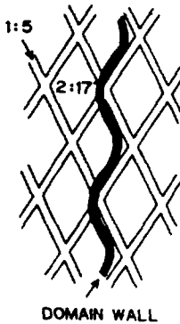
Fig. 6 Scheme of wall-pinning mechanism. 10)
