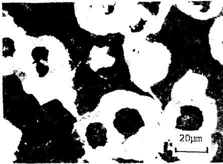
Fig. 2 Optical micrographs of as-cast ductile cast iron( \times 600 )
