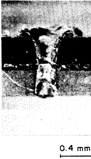
Fig. 4. Longitudinal section of SK-5/SUS304 plates (0.4/0.4mm) spot-welded under laser power 42.5J/pulse, pulse duration 3ms.
