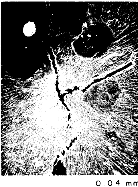
Fig. 9. Appearance of SK-5/PBS plates(0.2/0.4mm) spot-welded under laser power 30J/pulse, pulse duration 9ms.
