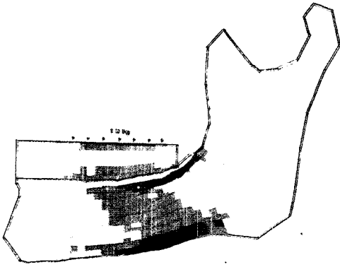
Fig. 24. Equivalent stress of structure with acrylic resin denture (P 3 -I).
