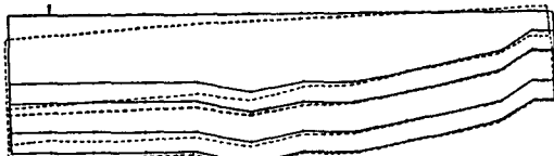
Fig. 9. Displacement of structure with resilient layer ( P_2 -III).
