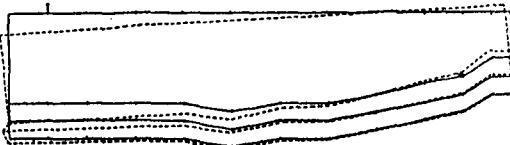
Fig. 8. Displacement of structure with resilient liner ( P_2 -II).
