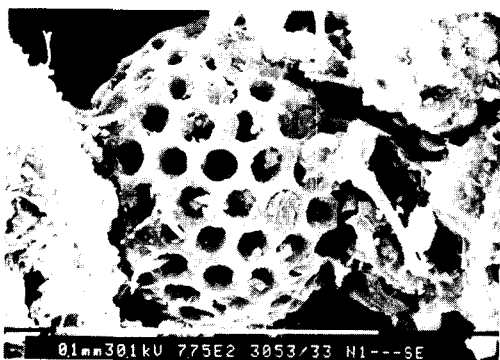
Fig. 4. Scanning electron micrograph for type A microlayer showing a radiolarian fossil and blades of todorokite.
