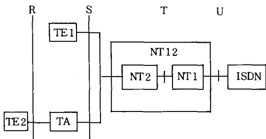
TE1 Terminal Equipment Type 1 (ISDN Terminal)
