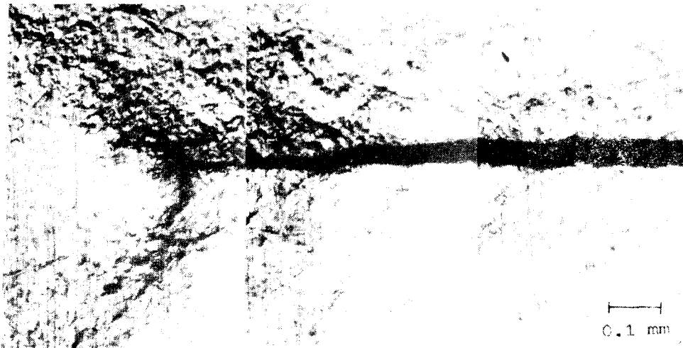
Photo. 2 Macro-graph of plastic deformation at crack tip
