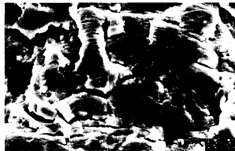
Photo.4 SEM fractograph of the fatigued surface of a weld metal (in room-temperature air, \Delta K=33MPa \cdot m^{1/2} , arrow indicates the direction of crack propagation)
