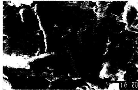
Photo. 1 SEM fractograph of the fatigued surface of a base metal (in room-temperature air, \Delta K = 33 \text{MPa}\cdot\text{m}^{1/2} , arrow indicates the direction of crack propagation)
