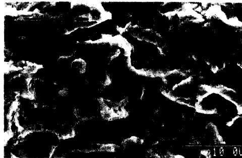
(b) Ahead of the corrosion fatigue crack tip (fatigue fractured in room-temperature air)
