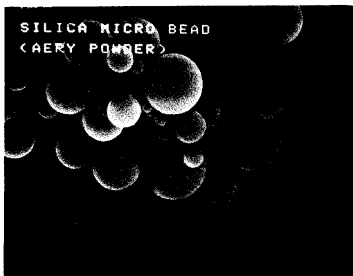
Fig. 1. Scanning electron microphotograph of silica spheres.
