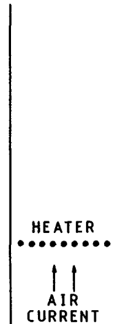
Fig. 1 The Rijke tube with heater wires
