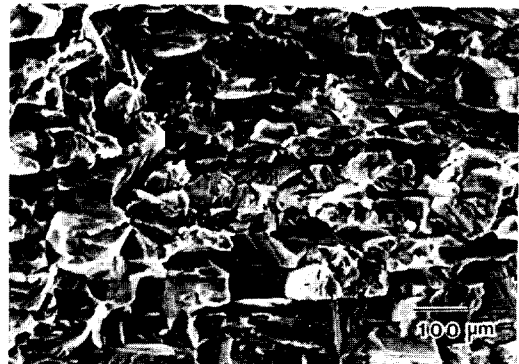
Photo. 10. SEM fractographs of SCC in base metal
