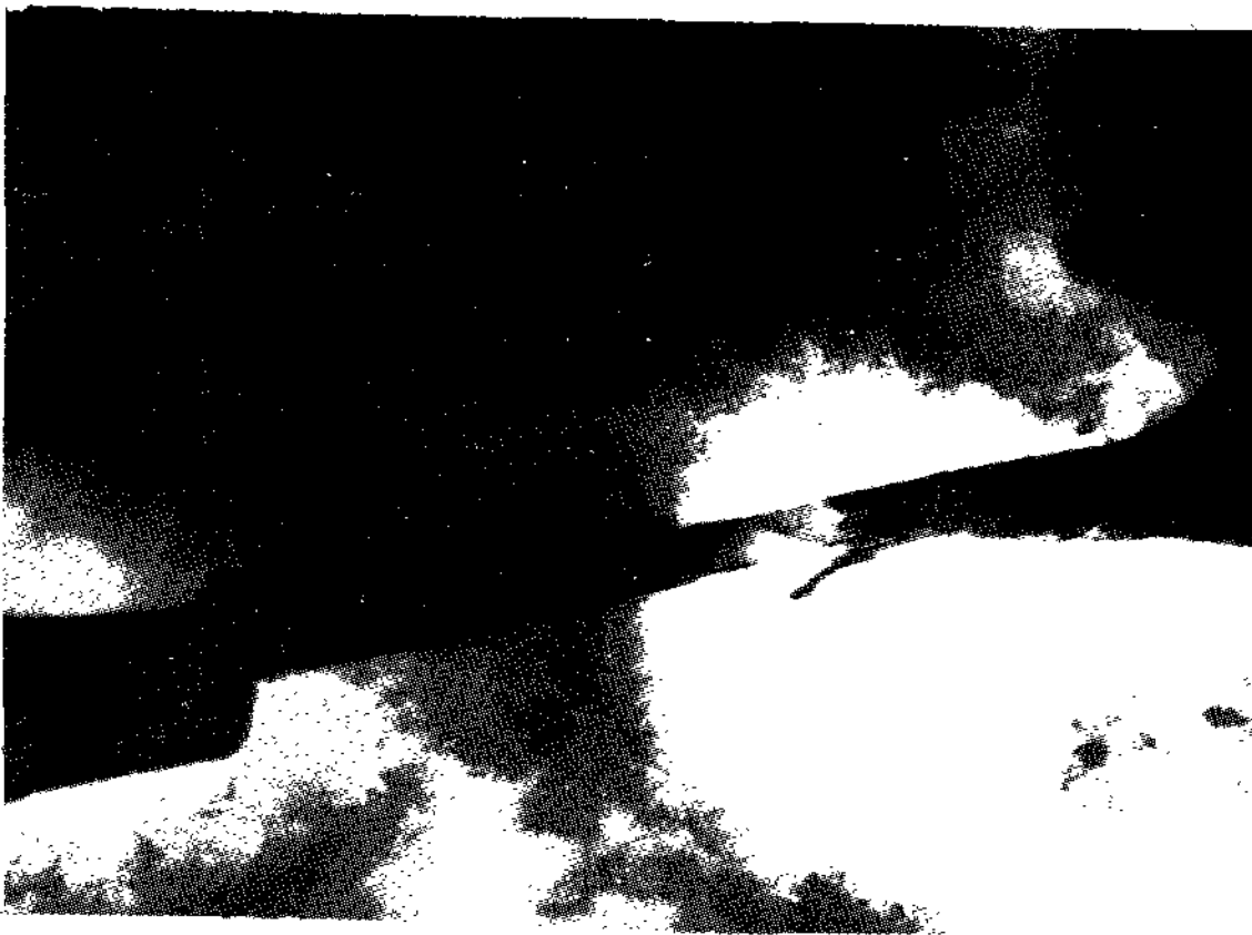
Fig.14. Eutectic silicon phase extracted from a 2.0% misch metal modified 356 aluminum alloy cast into a 1.25 in.D. graphite mold. Transmission electron microscope.
