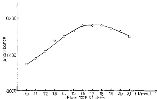
Fig. 2. The effect of acetylene flow rate on the absorbance of calcium ( 9.0 \times 10^{-5} M) in 0.05M HCl solution at constant air flow rate (7.7 l/min).
