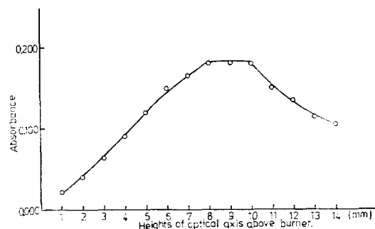
Fig. 1. The absorbance of calcium 9.0 \times 10^{-5}\text{M} at different height of optical axis above burner in 0.05\text{M} HCl solution.
