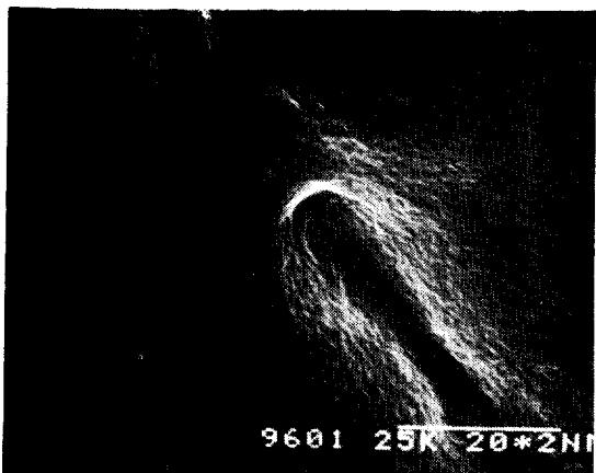
**Fig. 8.** Sanning electron micrograph of the surface habutae fiber (soaping,  $\times 15,000$ )
