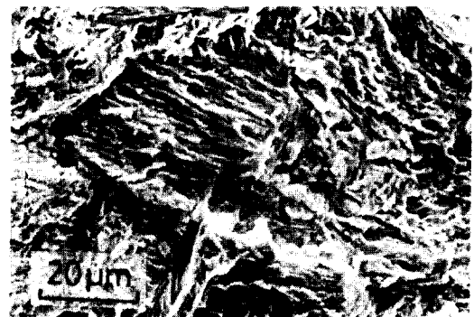
(b) number of cycle to fracturing 1.5 \times 10^6 , S_{max} = 17 \text{Kg/mm}^2
