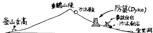
Figure. Prevention dyke of rock-slide. It was made as a counter-plan by the Busan Municipal Office after the accident of rock-slide at the slope of Mt. Seunghag.
