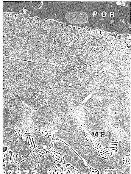
Fig. 15. Scanning electron microscopy of porcelain and alloy with lasing: POR, porcelain; HAZ, heat affected zone; MET, metal.
