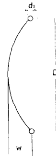
(b) 吸收材內形周邊裝荷 拋物形空中線 Rim loading on parabolic antenna with absorber.
