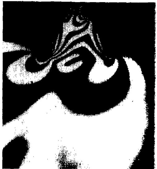
Fig. 2. Isochromatic lines of an internal gear tooth.
