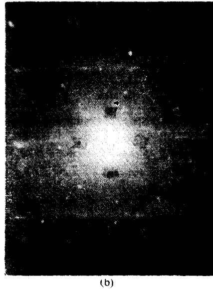
Fig. 13. Determination of Orientation on LiF Crystal (a) is a schematic figure of sample 8 and Growth Axis is [313] (b) is a Laue Back-Reflection Photograph on (001) Plane of Sample 8.
