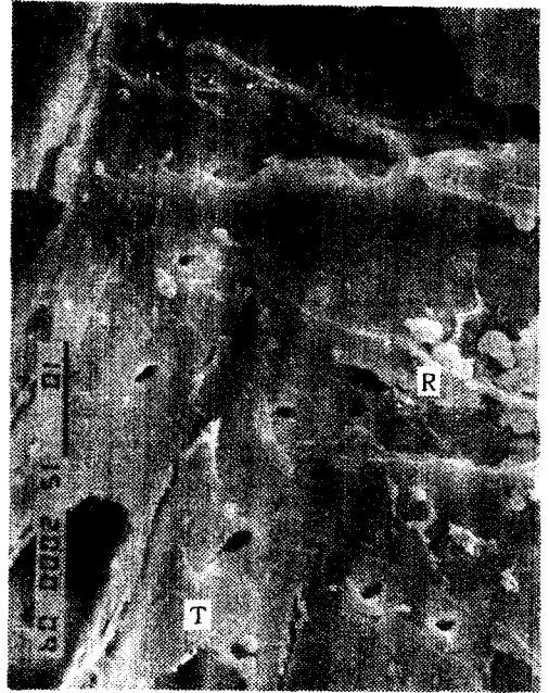
Fig. 8. Radial surface of compression wood, showing cross-field pit. Scanning electron micrograph (scale bar 10μm)
