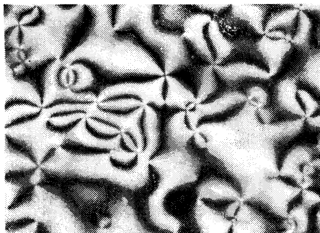
Figure 3. Photomicrograph of I_7 taken at 125°C. The sample was cooled down from 150°C at the rate of 3°C/min (original magnification; 150X).
