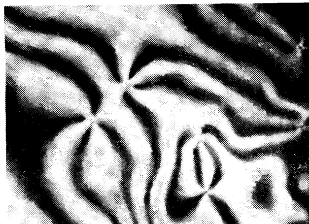
Figure 4. Photomicrograph of I_{12} taken at 130°C. The sample was cooled down from 150°C at the rate of 3°C/min (original magnification; 150X).
