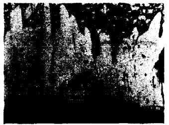
Photo.1. Microstructure of alloy layer produced by aluminizing treatment in molten aluminum bath at 730°C (x100).
