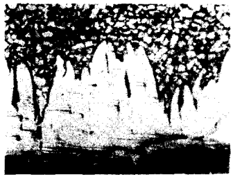
Photo.1. Microstructure of alloy layer produced by aluminizing treatment in molten aluminum bath at 730°C (x100).
