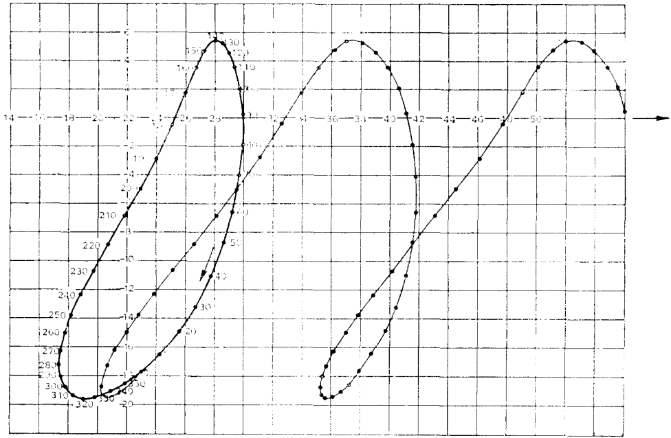
Fig. 11. Coupler curve of mechanism C relative to machine frame and ground.
