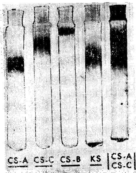
Fig. 1. Electrophoresis of mucopolysaccharides using procedure I. A current of 4 mA per gel column was applied in 0.03 % hexamine cobaltic chloride in 0.05 M sodium acetate buffer (pH 4.8) for 2 hrs.
