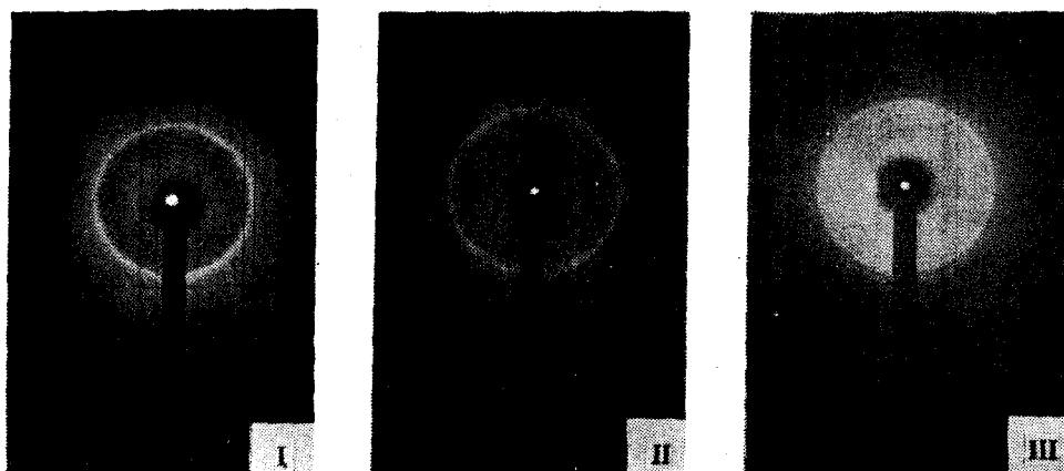
Fig. 5 X-Ray Diffraction Patterns of Sericin I, II and III
