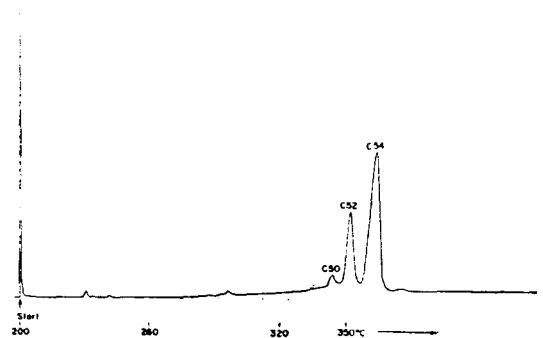
Fig. 5. Gas chromatogram of triglycerides in decuticled sesame oil (Sam Yang Oil Co.)
